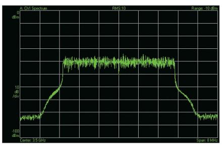
Figure 1. This basic spectrum measurement reveals much about an OFDM signal, though its untriggered averaging of a pulsed signal introduces some uncertainties. This measurement is good for determining the signal center frequency and approximate bandwidth, average power and flatness, and verifying the missing (normally untransmitted) center carrier.
