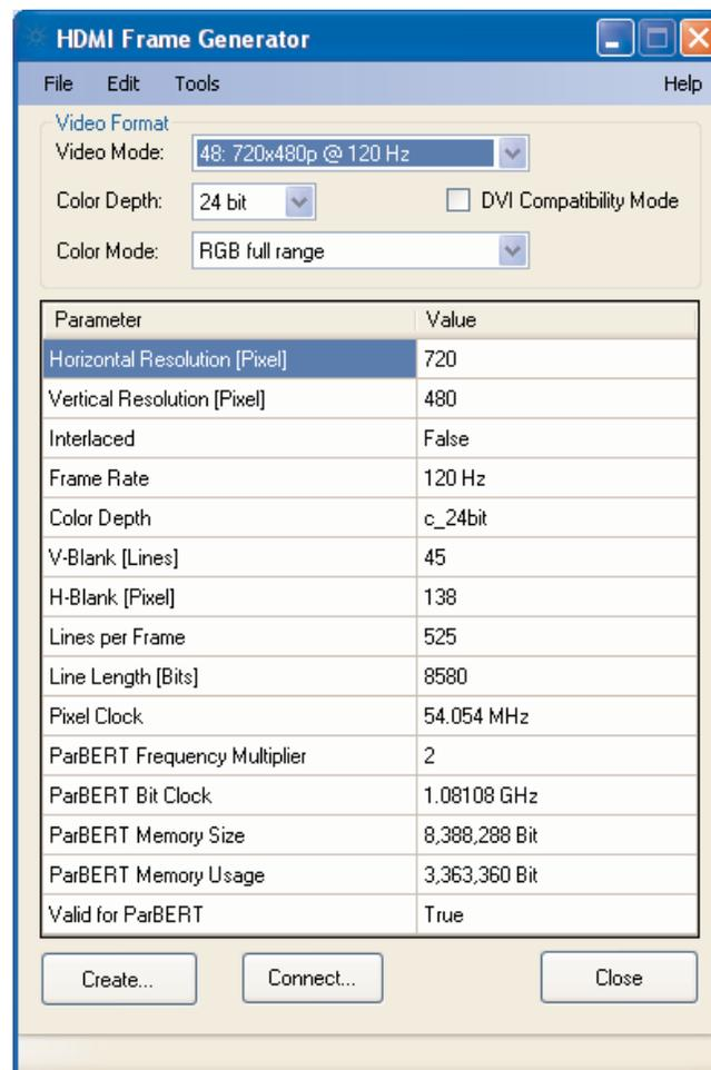
Figure 2: HDMI frame generator software
