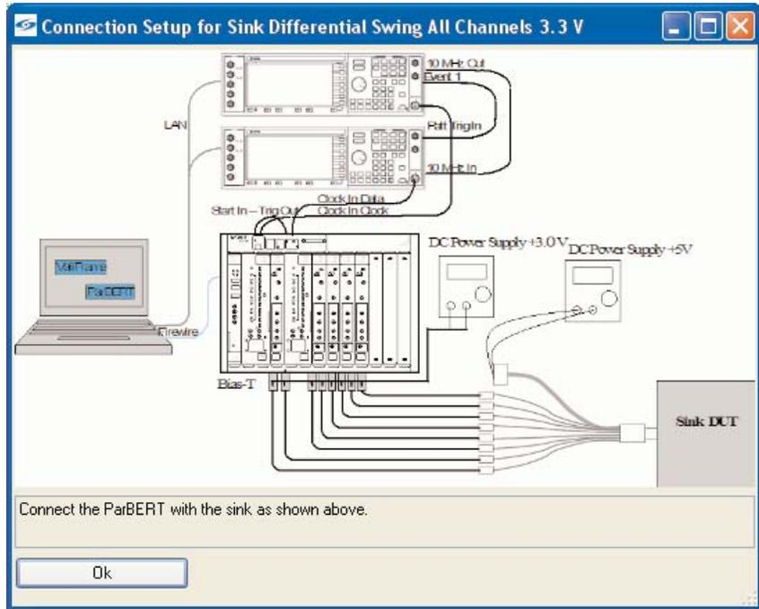
Figure 6: Sink test connection setup example
