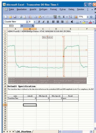
Figure 9: Source rise time test
