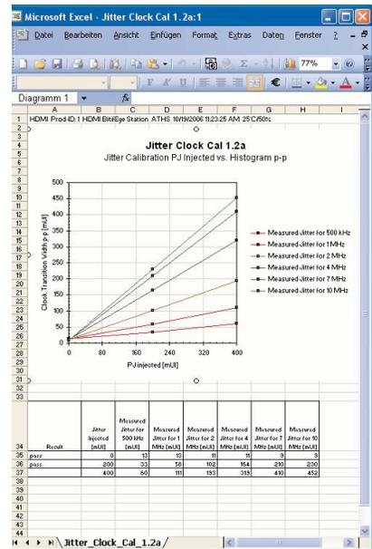
Figure 5: Clock jitter calibration results
