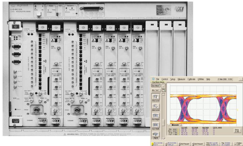
Figure 1: ParBERT 81250-based TMDS Signal Generator
