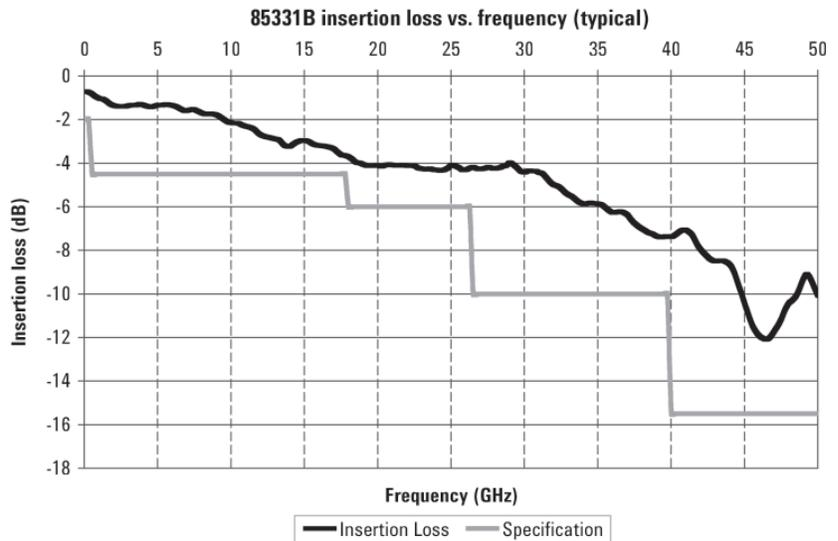
Figure 5. 85331B insertion loss vs. frequency (typical)
