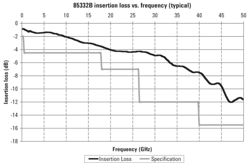
Figure 10. 85332B insertion loss vs. frequency (typical)
