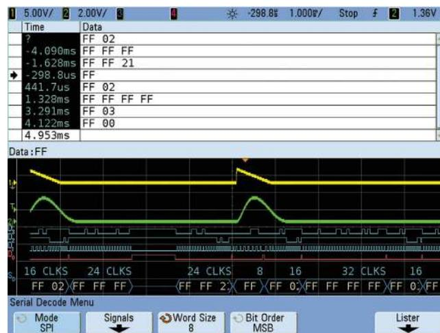
Figure 2. On-screen serial decode of SPI signals with time-correlated analog and digital waveforms capture by an MSO7104B.
