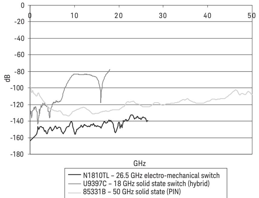
Figure 5. Electro-mechanical versus solid state switch isolation (typical)
