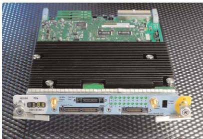
The Agilent Protocol Analyzer for PCIe 2.0
