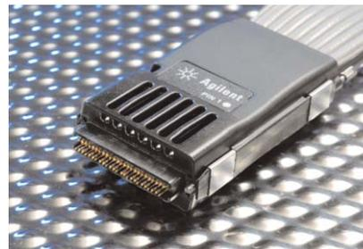
The Agilent Midbus 2.0 series of probes using soft touch technology
