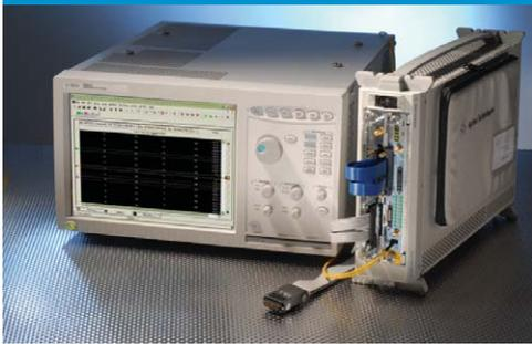
The Agilent Protocol Analyzer and Logic Analyzer with the P2L gateway cable
