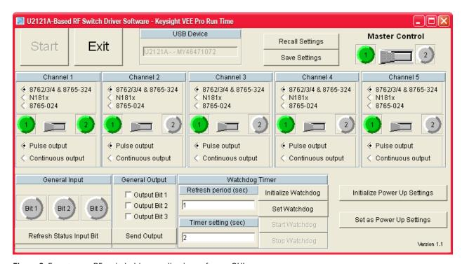
Figure 2. Easy-to-use RF switch driver application software GUI
