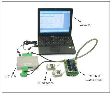
Figure 1. Example of a general RF test system
