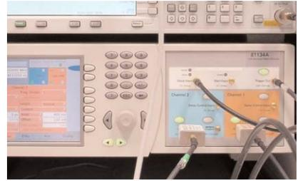
Figure 3: Transition time converters connected to the generator output.
