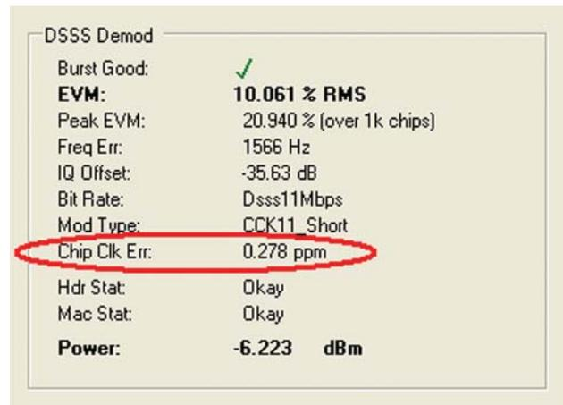
Figure 9. Demod measurement showing the chip clock frequency error result
