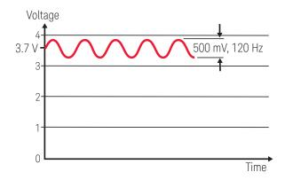
Figure 1. Example test waveform powering DC-to-DC converters
