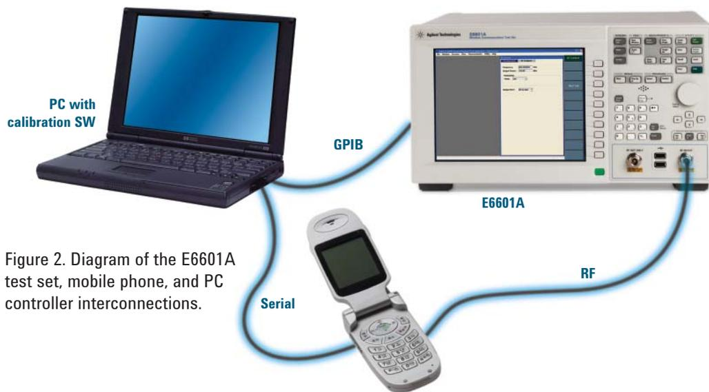
Figure 2. Diagram of the E6601A test set, mobile phone, and PC controller interconnections.
