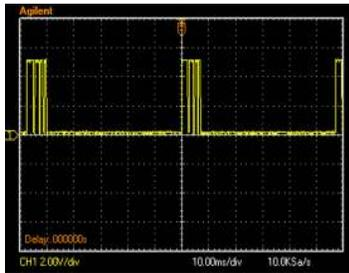
Figure 4 A 5 V Irregular Pulse Signal
