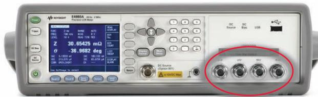
Figure 5. Test ports of the E4980A
