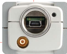
Built-in triggering port for synchronization with external instruments or events
