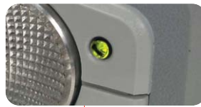
LED indicator for PC communication
