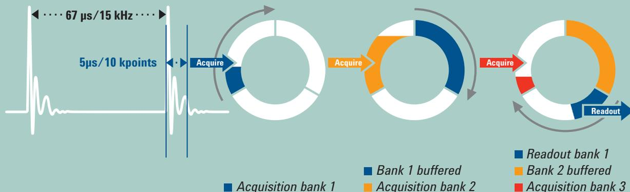
Figure 1. Simultaneous multibuffer acquisition and readout mode example
