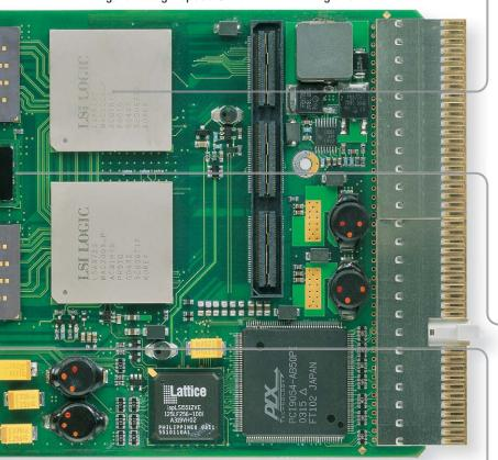
Figure 1: High-speed U1062A-002 PXI digitizer
