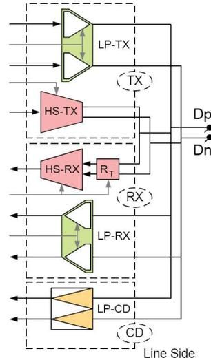
Figure 2: Electrical Functions of a fully featured D-PHY transceiver
