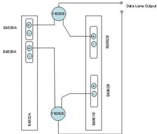
One low speed lane is 2 x E4838A    One high speed lane is 2 x E4862B
