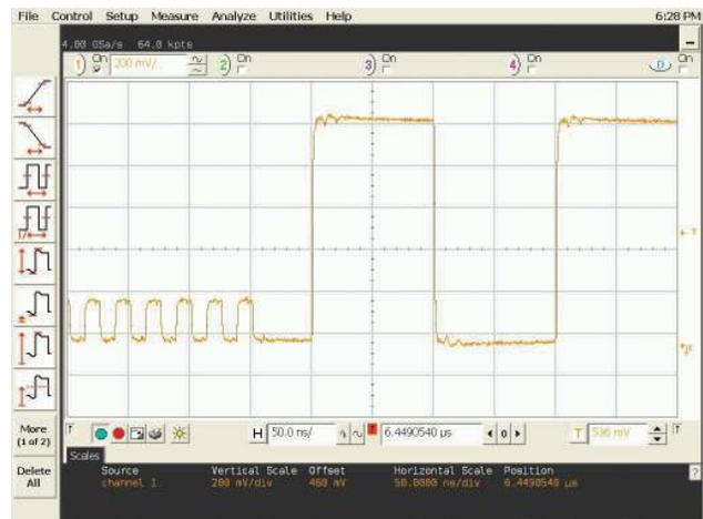
Figure 11: Zoom into the bit level of the D-PHY stimulus signal switching between HS and LP mode
