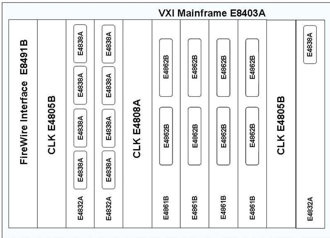
Figure 6: 81250A ParBERT configuration for testing a two lane phy configuration
