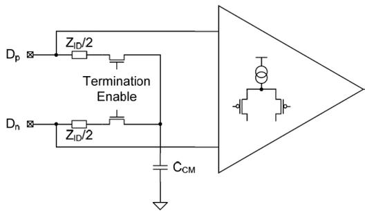
Figure 3: HS Receiver implementation including switchable termination
