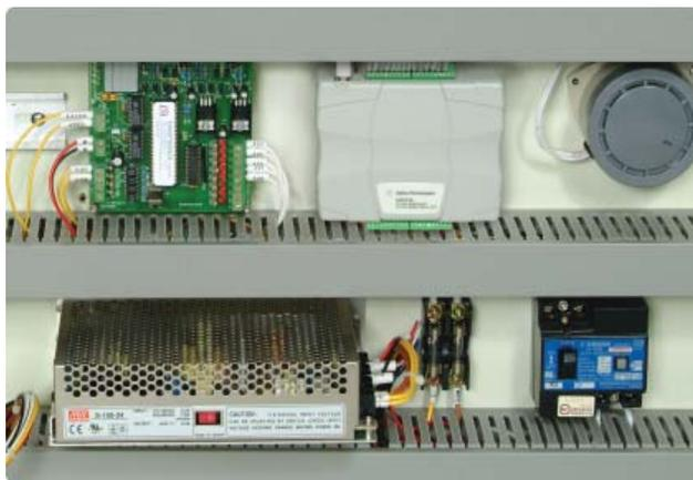
Figure 2. The U2100A is incorporated in the automated handler machine.
