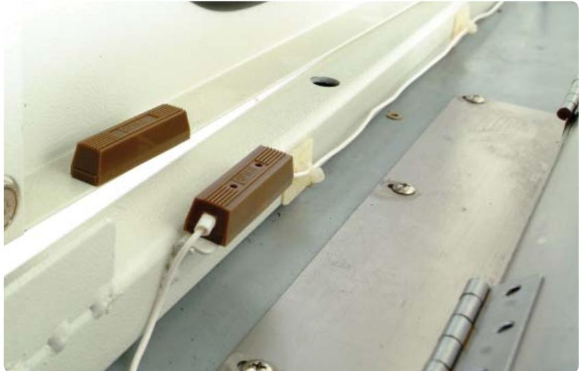
Figure 6. The magnetic sensors are mounted to the test system door.
