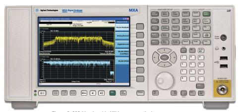
Figure 2. 802.11g signal in VXA vector analysis measurement (with external trigger, 20 kHz RBW and auto-scale on Trace 1).
