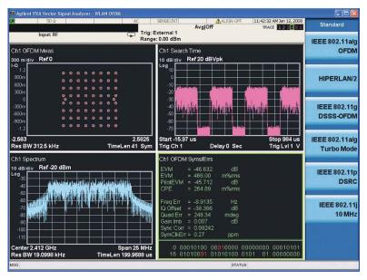
Figure 4. 802.11g WLAN OFDM modulation analysis in default quad view: Trace 1 (upper left), IQ constellation; Trace 2 (lower left), spectrum; Trace 3 (upper right), search time, Trace 4 (lower right), Symbol/error table with demod bits
