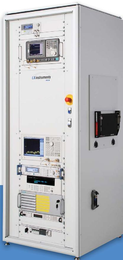
*The LXinstruments system for testing automotive antenna amplifiers*
