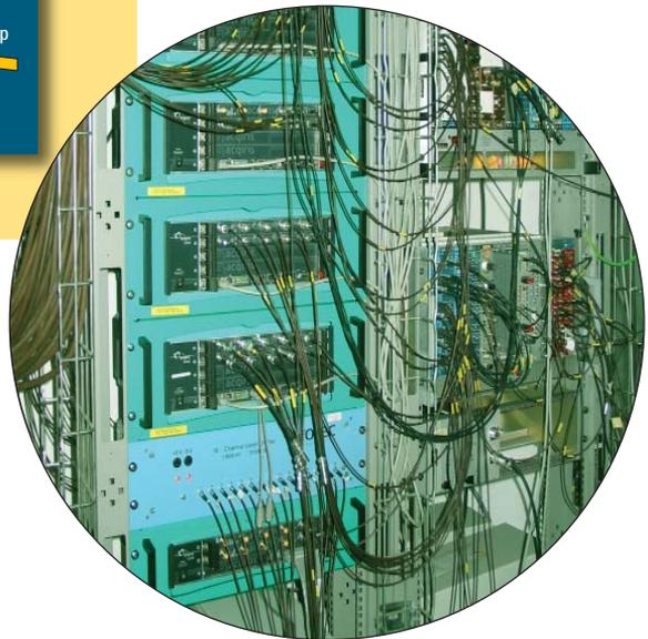
Figure 3. High-speed data acquisition system
