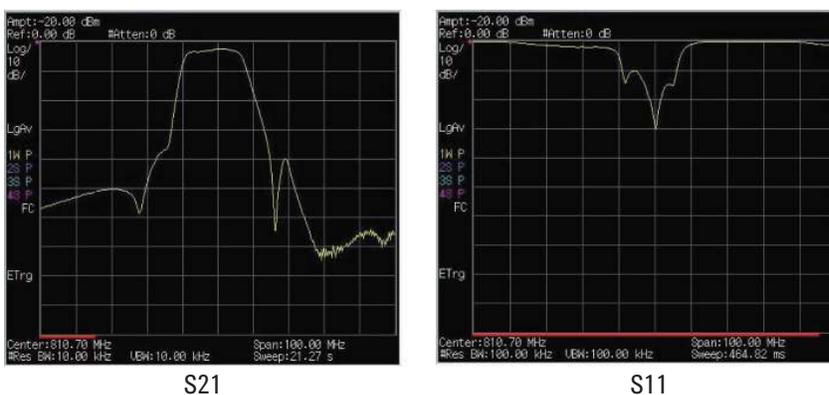
Figure 4. Screenshot of filter  $S_{21}$  and  $S_{11}$  measurement
