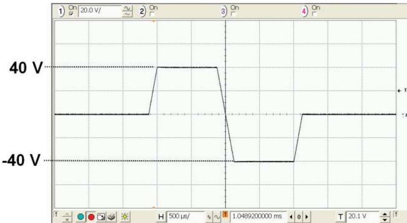
Figure 8. The HV-SPGU can output a three-level pulse with  $\pm 40$  V output swings.
