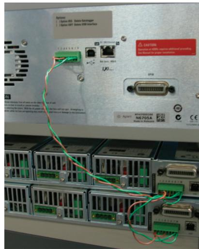
Figure 3b. Multiple mainframe wiring
