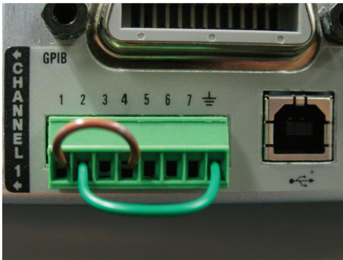
Figure 3a. 8-pin digital port connector wiring for single mainframe
