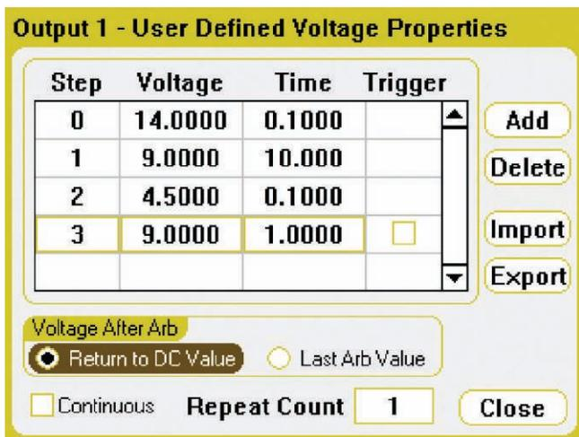
Figure 3. N6705A User Defined Voltage entry screen waveform
