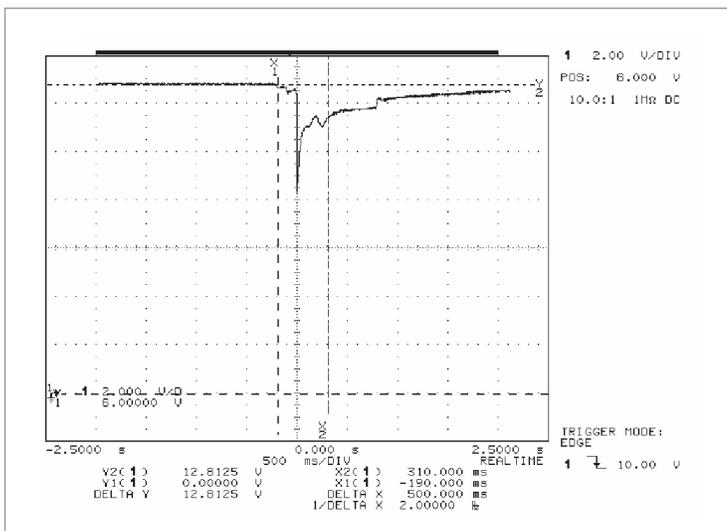
Figure 1. Power system transient due to starter motor crank
