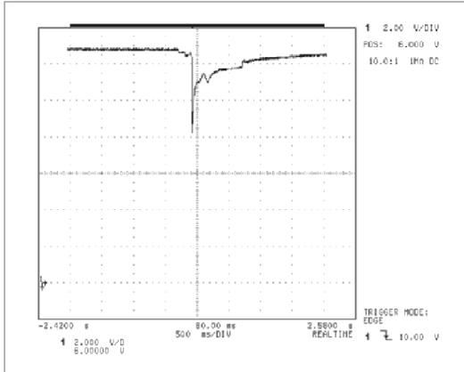
Figure 8. Original transient captured by scope
