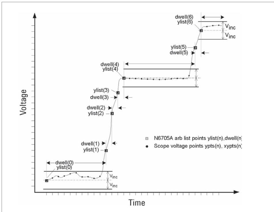
Figure 5. Compress 30 scope data points (ypts, xpts) to 7 voltage/dwell data points (ylist, dwell)
