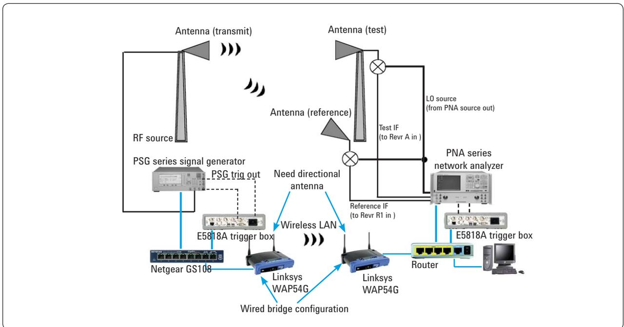
Figure 15. Long distance system synchronization via wireless LAN
