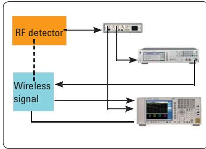
**Figure 10.** RF detector to E5818A
