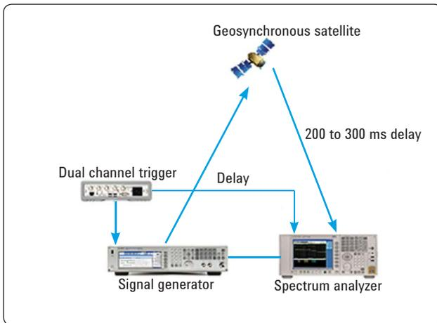
**Figure 12.** Near field measurement synchronization
