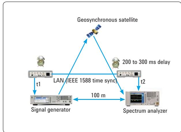
**Figure 13.** Far field measurement synchronization
