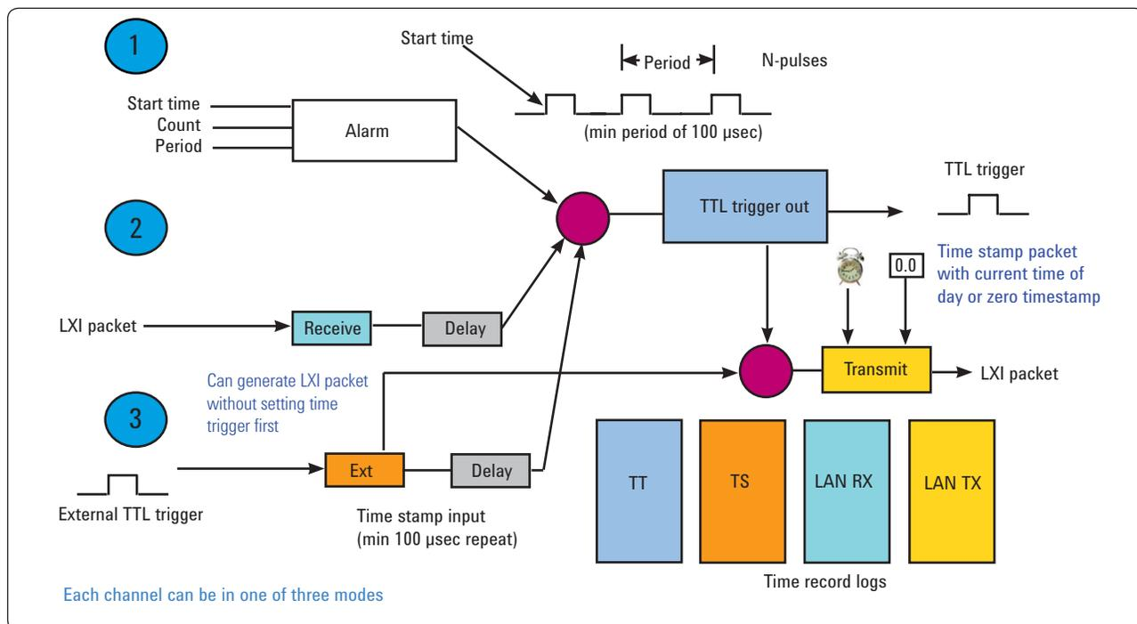
Figure 1. Three major modes that cause output trigger
