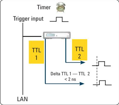
Figure 5. Synchronized triggering events
