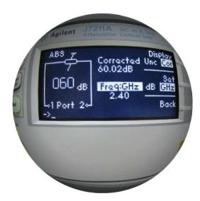
Figure 5. LCD display of Agilent Attenuation Control Unit
