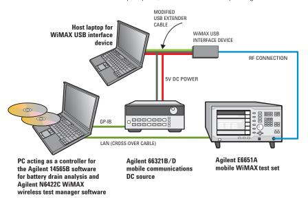
FIGURE 2: WiMAX WWAN USB device automated test example
