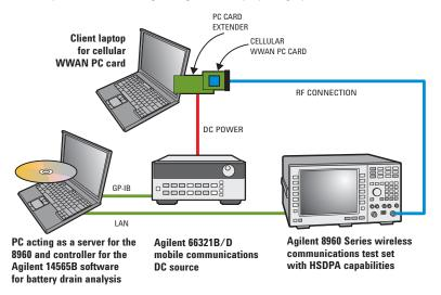
FIGURE 1: HSDPA WWAN interface PC card current drain test example
