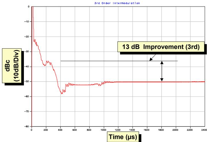
Adaptive RF Predistorter Using Rectangular Coordinate Work Function
