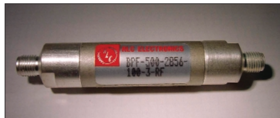
▲ Figure 9. Commercial tubular bandpass filters from K&L Microwave (top) and RLC Electronics (bottom).
