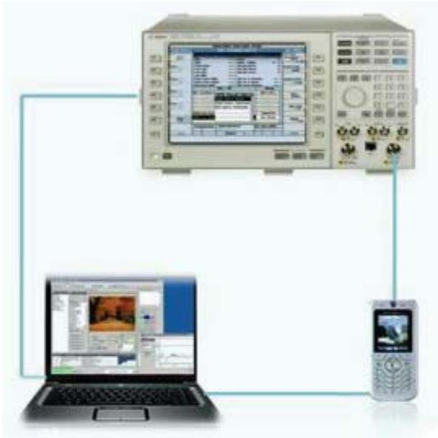
Figure 1: Test mode BER and MS calculated BER without a signaling connection or TCH loopback will reduce Rx test times
