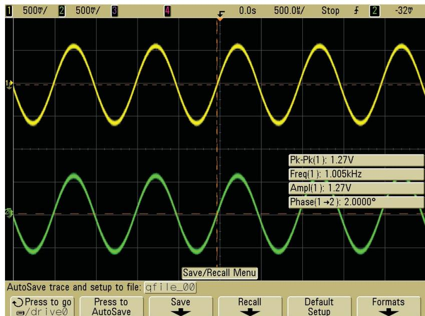
Figure 4. Oscilloscope with built in Vp-p and phase relationship measurement
