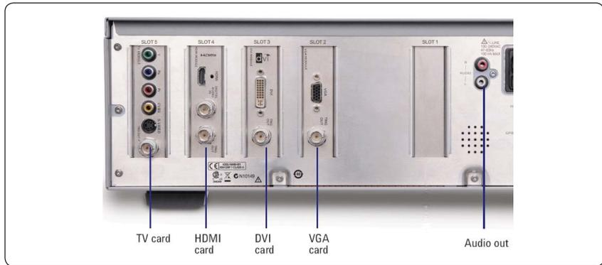
Figure 3. U8101A display tester with configurable plug-in cards
