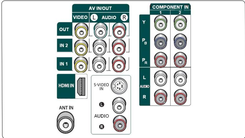
**Figure 1.** Typical types of TV connectors
