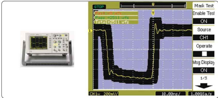
**Figure 5.** The DSO3000 Series two-channel oscilloscopes with mask test feature that automatically compares incoming signals with predefined mask (limits) and indicates fail or pass
