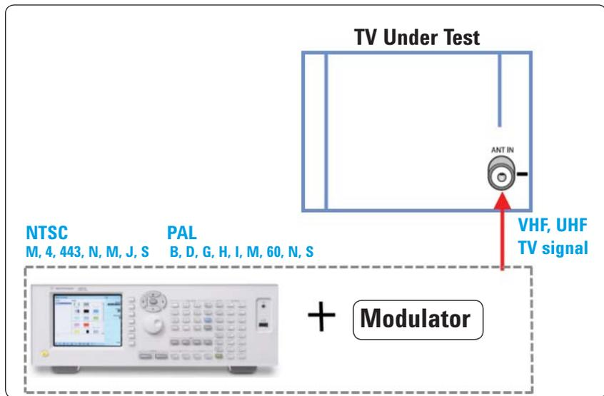
**Figure 6.** Antenna RF input test setup
