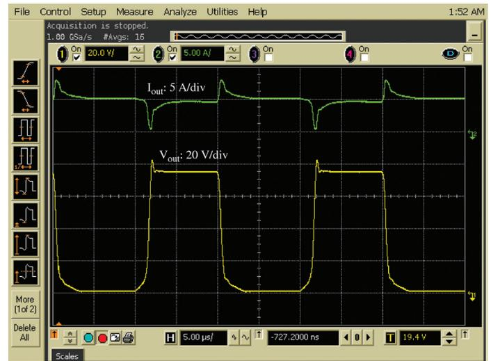
Figure 3. Keysight E4362A SAS output voltage and current waveforms (shunt switching at 50 kHz)
