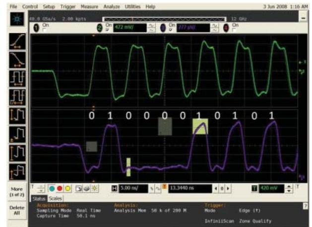
Figure 2: Using the InfiniiScan zones, a condition is set to track a specific DQ pattern of “01000010101”
