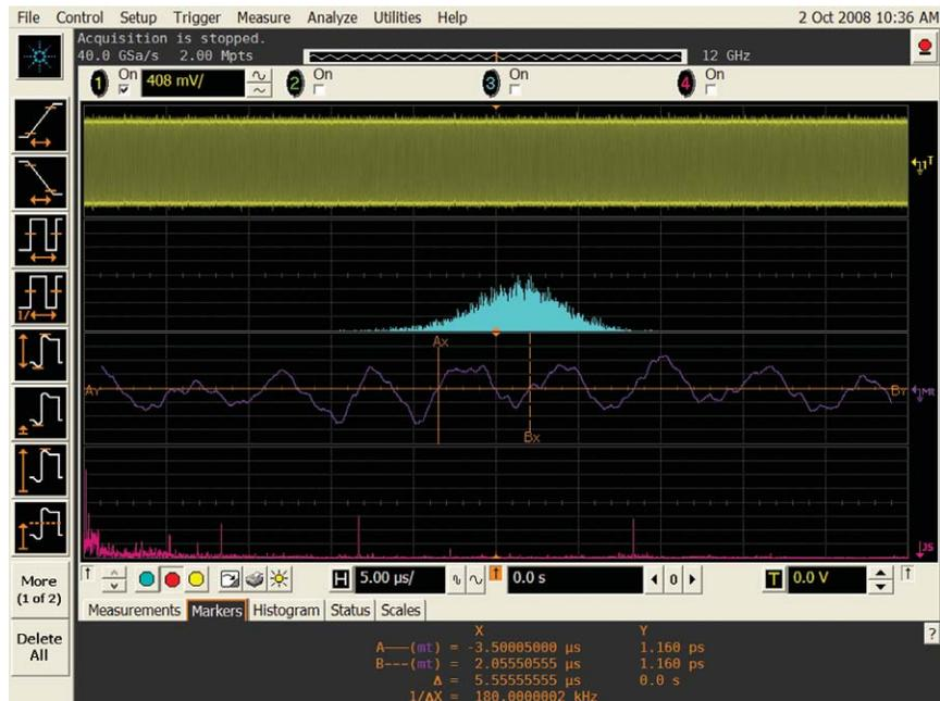
**Figure 6.** EZJIT lets you observe and measure the low-frequency jitter. Again the spectrum can help identify sources of jitter from frequency components. The low frequency with jitter of 180 kHz is due to a nearby switching power supply.
