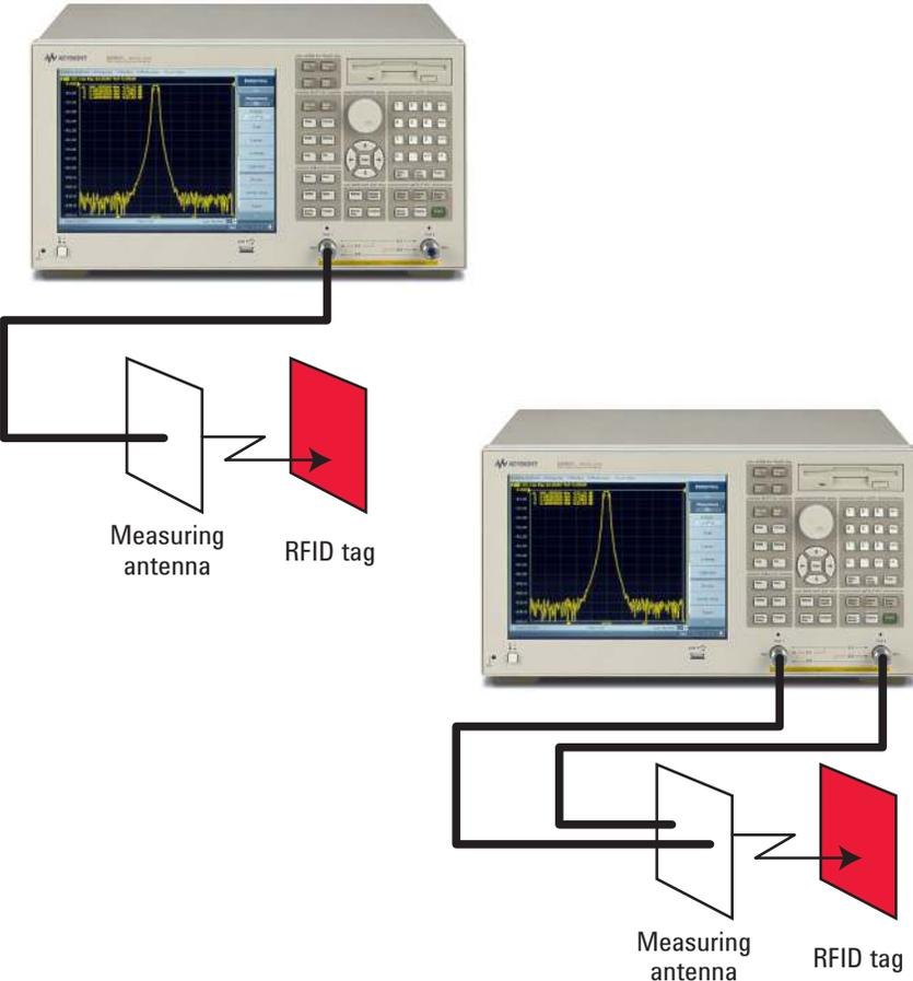
Figure 1. Measurement setup with reflection or transmission measurement
