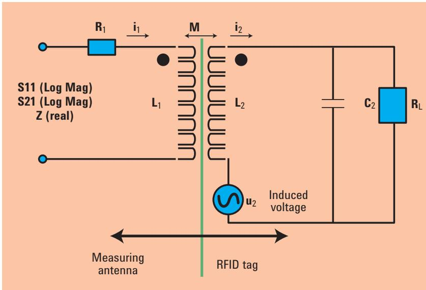
Figure 2. RFID tag electric circuit diagram
