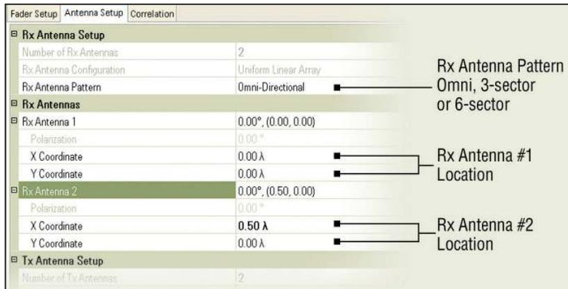
Figure 3. All antenna parameters affect channel correlation and therefore must be modeled using the antenna parameter setup menu shown here.
