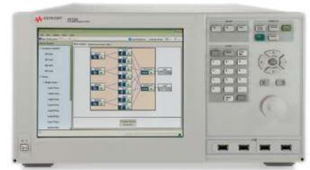
Figure 1. The N5106A PXB Baseband generator and channel emulator provides up to 4 baseband generators (BBGs), 8 faders, the industry's widest bandwidth of 120 MHz, custom MIMO correlation settings (e.g., predefined channel models, antenna pattern and correlation matrix), and supports testing and troubleshooting of 2x2, 2x4, and 4x2 MIMO.
