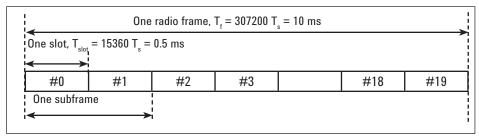
Figure 3. LTE frame structure type 1 (TS 36.211 V8.30)
