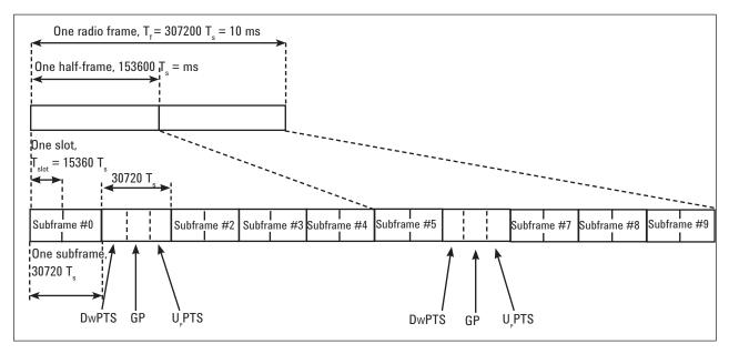
Figure 4. LTE frame structure Type 2 (5 ms switch-point periodicity) (TS 36.211 V8.20)
