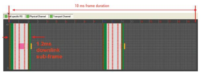
Figure 6. Sub-frame duration 1.2 ms of downlink signal captured with N7625B Signal Studio software
