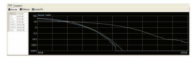
Figure 11. Waveform CCDF calculates the CCDF and peak-to-average ratio using the entire LTE-TDD waveform (with downlink signal off and uplink signal on)
