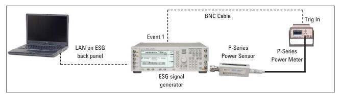
Figure 5. P-Series power meter and ESG signal generator setup diagram
