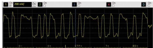
Figure 2. Example of embedded decode of 8B/10B symbols
