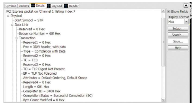
Figure 6. A Details Tab clearly shows the Physical, Data Link and Transaction Layers of a high speed protocol
