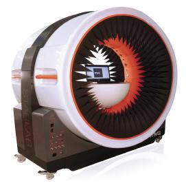
circumference of a support structure. The DUT is placed at the center of the support structure and measurements are made by electronically scanning the probe array in elevation and by rotating the DUT 180° in azimuth. By electronically scanning the multi-probe array the number of mechanical movements is minimized reducing significantly the time required to make your antenna measurements.
