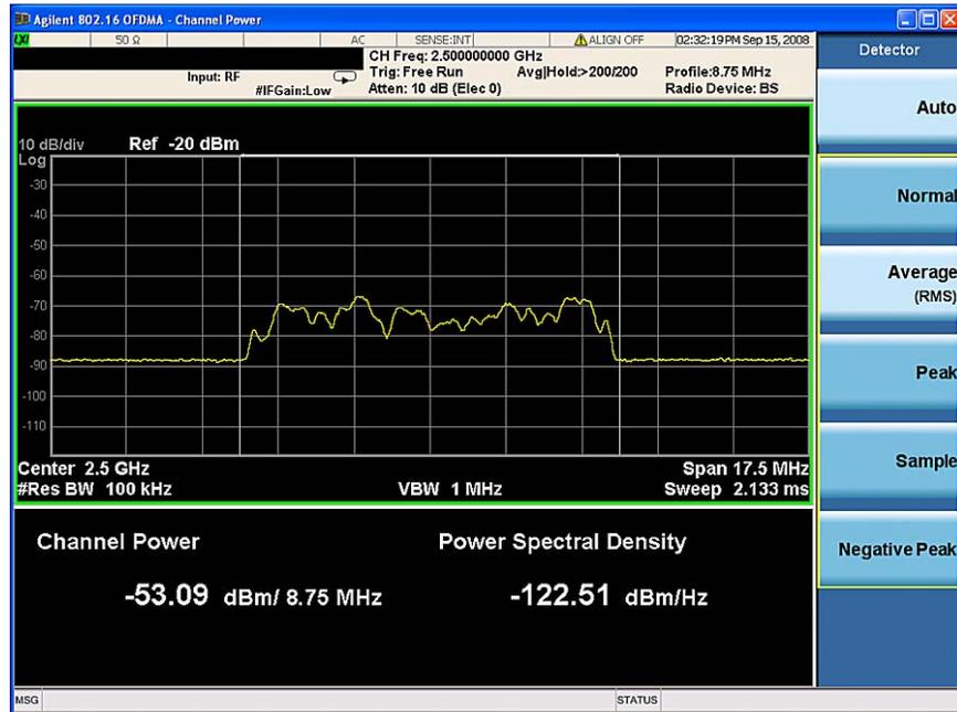
Figure 7. RF spectrum for Pedestrian B fading.
