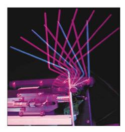
Semi-rigid Cable Automatic Bending Process
