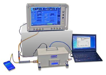
Load pull is an ideal solution for measuring the performance of mobile phones under real-world conditions. In the real world mobile phones have to operate even with a lost or damaged antenna, in a tunnel or locker, when held close to the body or when in a pocket surrounded by coins. All of these conditions create non-ideal, non-50 ohm RF environments and designers and manufacturers have to demonstrate that their products can continue to work in these situations.
