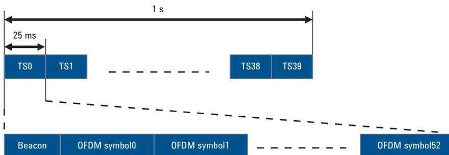
Figure 3. Frame structure.
