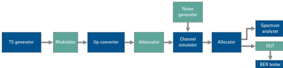
Figure 4. Block diagram for carrier-to-noise ratio threshold under fading environment.
