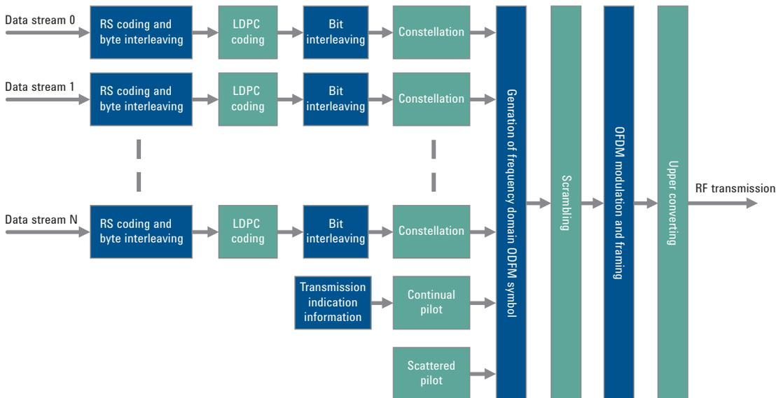
Figure 1. CMMB block diagram.
