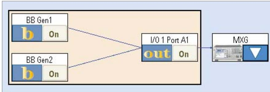
Figure 15. PXB configuration for interference testing.
