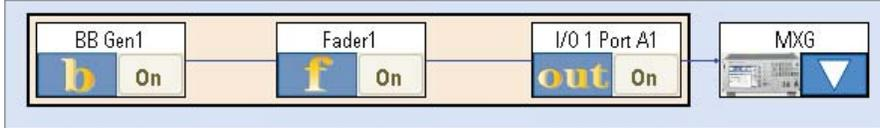
Figure 12. PXB configuration for multipath fading testing.
