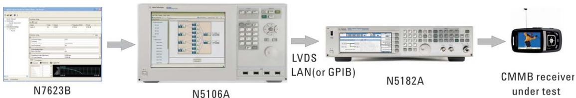
Figure 5. Conformance testing system setup.
