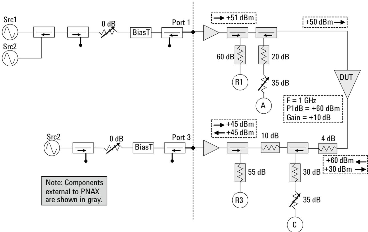
Figure 5. +60 dBm amplifier setup
