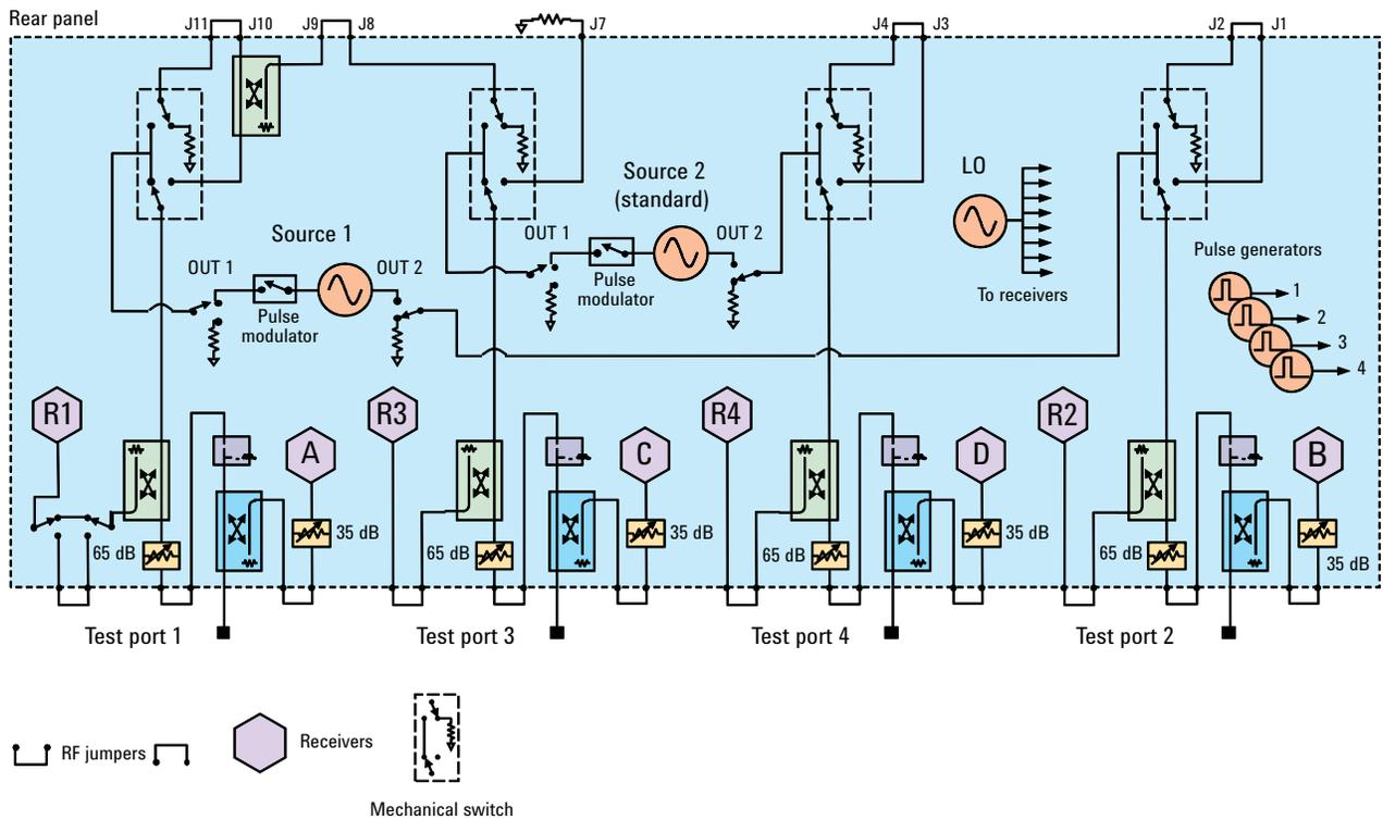
Figure 1. PNA-X N5242A Option 423 Test Set Block Diagram
