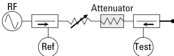
The cables connected to the attenuator should be kept as short and stable as possible to minimize measurement drift.
