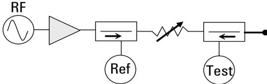
When measuring low gain devices, a pre-amplifier may be added to PNA-X port-1 to increase the DUT input power. As a general rule of thumb, the pre-amplifier's harmonics should be about 20 dB below the maximum main tone at the DUT input to avoid stimulating nonlinear behavior in the DUT which cannot be corrected by the NVNA.
