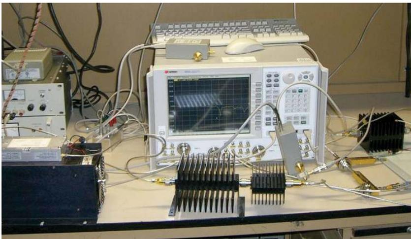
Figure 7. Photograph of test setup for 100 W amplifier
