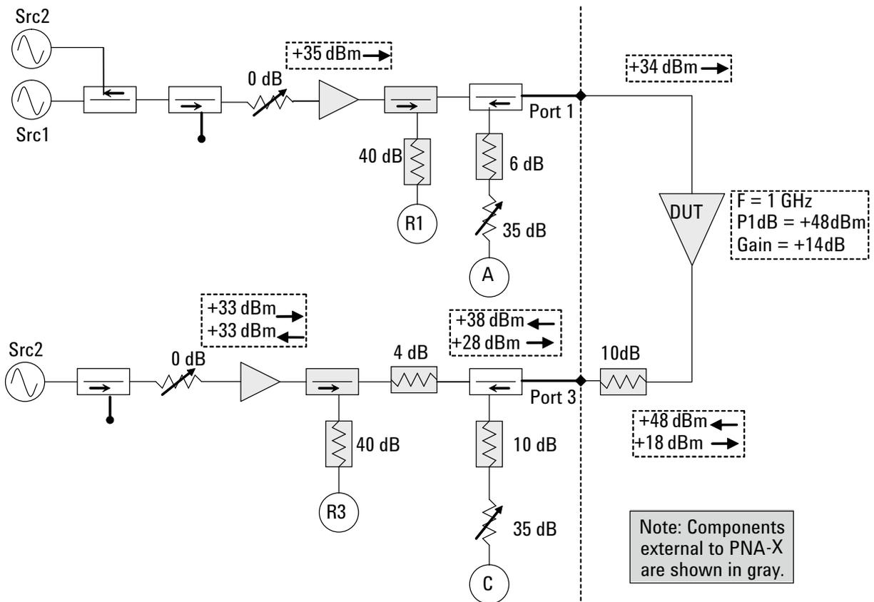
Figure 4. +48 dBm amplifier setup
