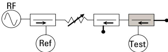
Note that the PNA-X test coupler arm rolls off at 20 dB/decade for frequencies below 700 MHz, so that the typically -15 dB coupling factor is reduced to -52 dB at 10 MHz. If an external test coupler is added which doesn't exhibit this roll-off, then the dynamic range at low frequencies will be improved.
