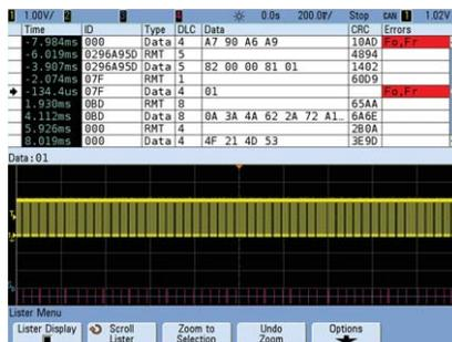
Notice that when scrolling through the decode list that the waveform in the lower half of the display "tracks" with direct time-correlation.
