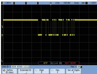
Notice the flashing red "ERR" error message in the decode trace. With the scope industry's only hardware-based serial decoding, InfiniiVision scopes capture infrequent serial communication errors that other scope miss
