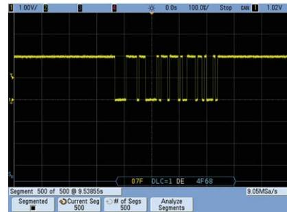
Segmented Memory acquisition conserves valuable acquisition memory by only capturing important segments of input signals. This is useful for low duty cycle signals such as laser pulses, and packets of serial data.
