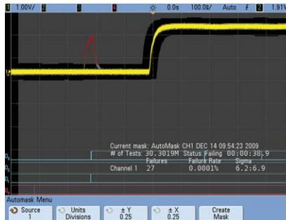
With the scope industry's only hardware-based mask testing, InfiniiVision scopes can test up to 100,000 waveforms/sec based on pass/fail boundaries.
