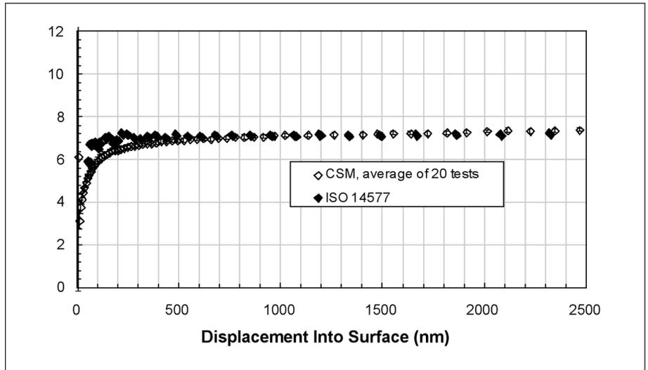
Figure 4. Hardness of Pyrex as a function of surface penetration using two test methods.
