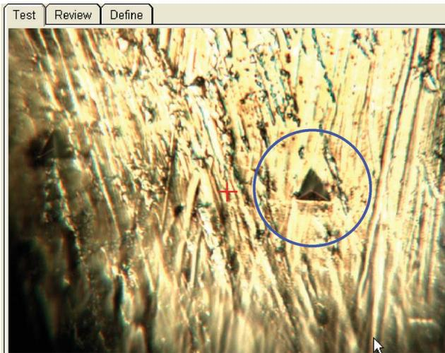
Figure 5. Residual impression from 650 mN indent on the TiN coating (40X objective).
