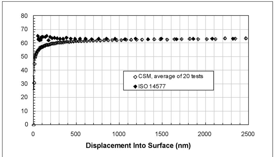
Figure 3. Modulus of Pyrex as a function of surface penetration using two test methods. Area function for this Berkovich diamond tip is  $A(d) = 24.5037d^2 + 281.7d$ , where  $d$  is the distance along the diamond axis from the apex to the contact plane.
