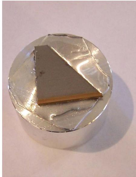
Figure 1b. Utility blade as mounted for testing in the G200.
