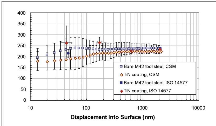
Figure 6. Modulus vs. penetration depth for coated and uncoated regions of utility blade. Error bars span one standard deviation.
