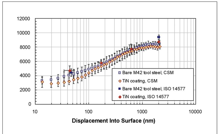
Figure 8.  $S^2/P$  vs. penetration depth for coated and uncoated regions of the utility blade. Lower value of this parameter means greater resistance to damage. These results do not reveal any mechanical advantage conferred by the TiN coating.
