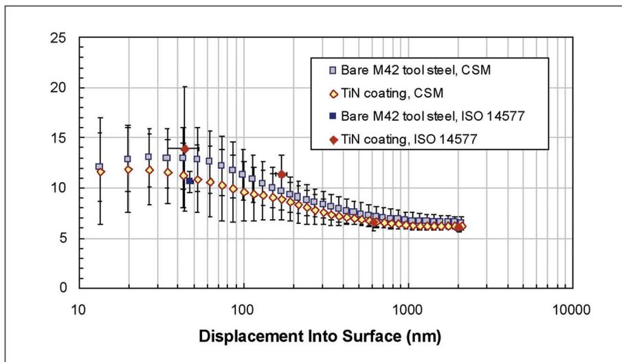
Figure 7. Hardness vs. penetration depth for coated and uncoated regions of utility blade. Error bars span one standard deviation.
