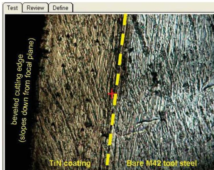
Figure 2. Image of test surface (10X objective). Eight residual impressions from tests on the TiN coating are visible.
