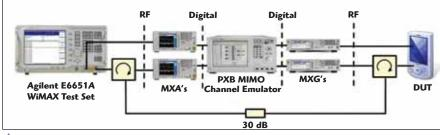
igtriangle Fig. 1 Equipment set-up for measuring receiver performance.
