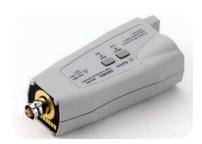
The N5477A sampling oscilloscope adapter makes the InfiniiMax III probing system fully compatible with the Infiniium 86100C DCA-J sampling oscilloscope. Previously the DCA-J was limited to 13 GHz of probing, but with the N5477A, the DCA-J now has 30 GHz of probing, increasing its performance and flexibility. To use the InfiniiMax III+ probe on sampling oscilloscopes, order the N1022B probe adapter and the 1143A probe offset control and power module.
