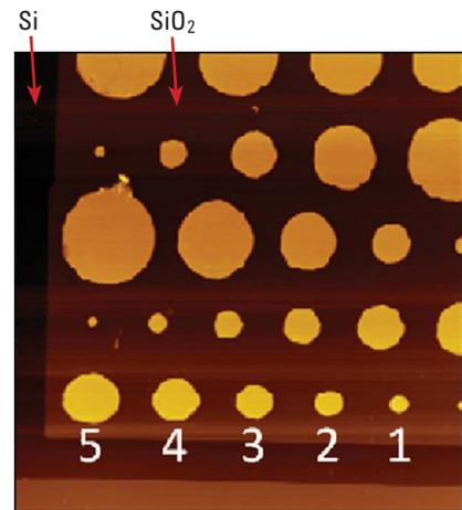
Figure 1. AFM topography image of NIST capacitance standard.
