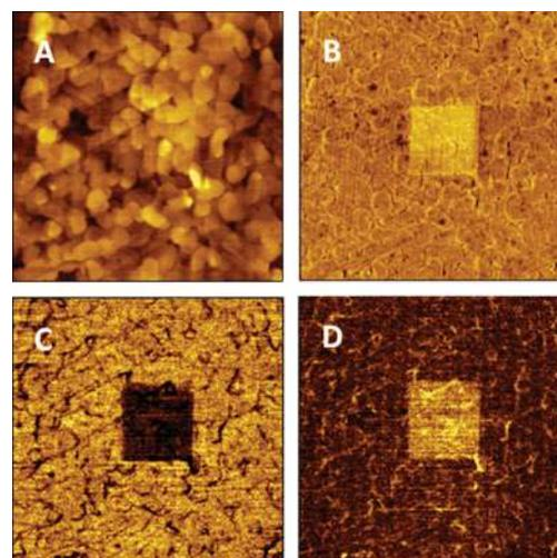
Figure 6. SMM imaging of a C18/C10 SAM structure on Au(111) surface: A) topography, B) friction, C)  $S_{11}$  amplitude, and D)  $S_{11}$  phase.
