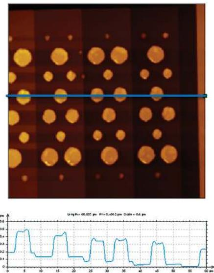
Figure 4. Standard capacitance structure for SMM calibration, which consists of Au pads of well defined area deposited on SiO<sub>2</sub> films of precise thickness.
