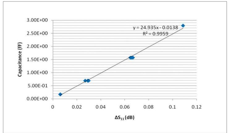
Figure 3. A linear plot of Capacitance against  $\Delta S_{11}$  with the slope being the calibrated transfer coefficient of the SMM system.
