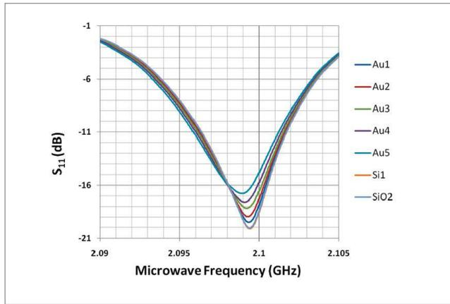
Figure 2. Reflection coefficient  $S_{11}$  versus frequency plot measured on different Au pads, Si, and SiO<sub>2</sub>.
