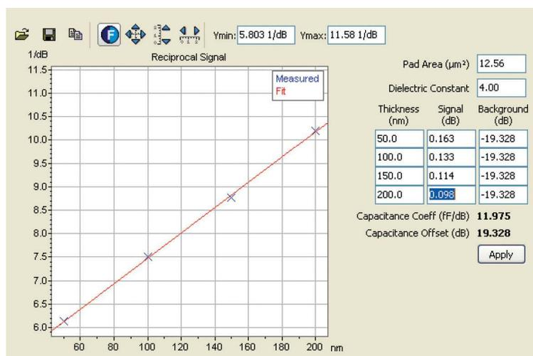
Figure 5. Screenshot of the capacitance calibration GUI in PicoView. The transfer coefficient of the SMM system is calculated from the linear plot of  $1/\Delta S_{11}$  vs  $d$ , the thickness of the  $\text{SiO}_2$  layer.
